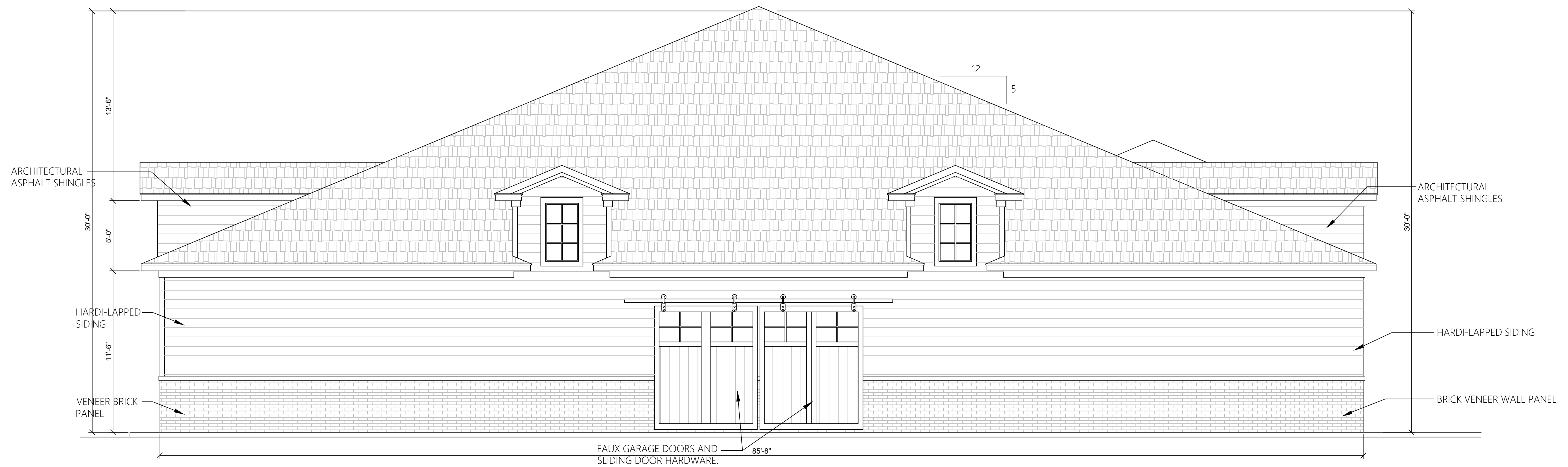
1 A02 PRELIMINARY REAR ELEVATION SCALE: 1/4"=1'-0"
