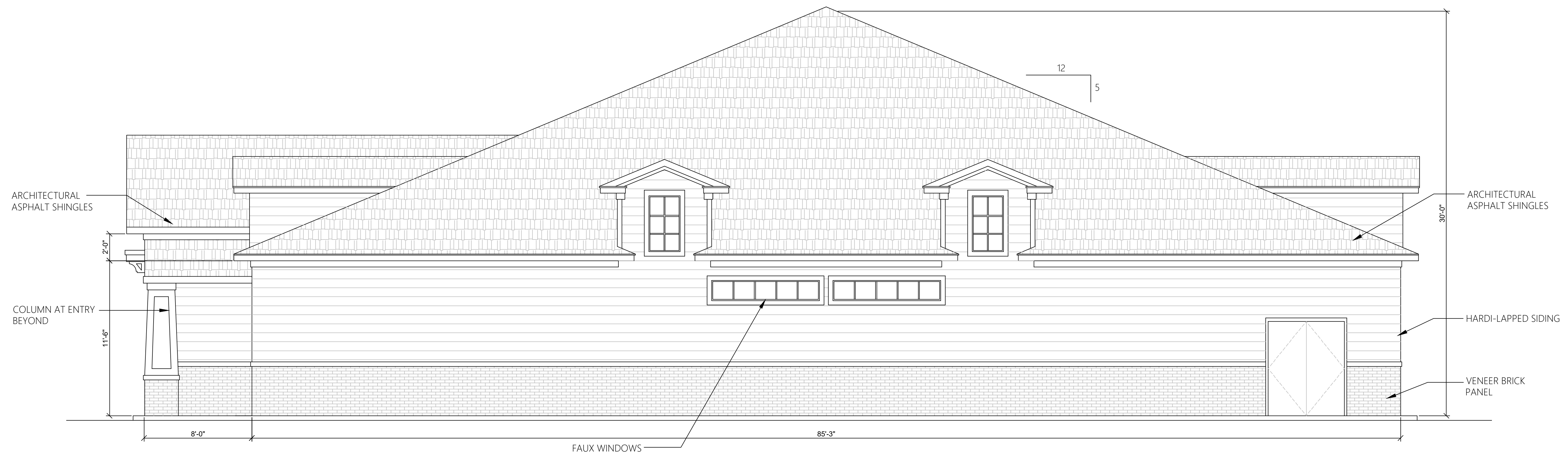
2 A02 PRELIMINARY RIGHT SIDE ELEVATION SCALE: 1/4"=1'-0"
